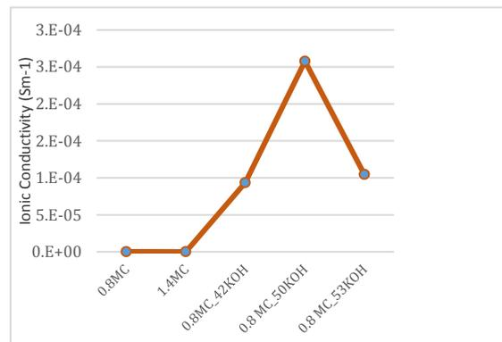
Figure 4: Result for ionic conductivity test  $\text{Sm}^{-1}$  of MC-KOH
