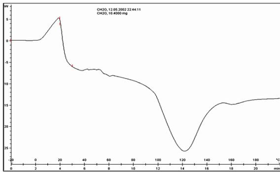
Figure 4: DSC of calamansi lime pectin from water solvent residue
