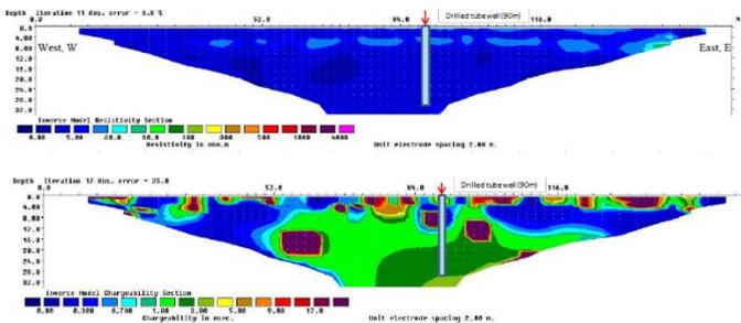
Figure 3: Electrical resistivity and chargeability tomography results
