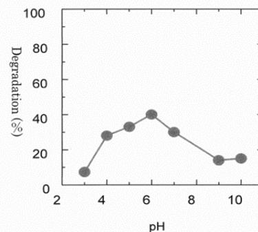
Figure 4: Effect of pH value on photocatalytic degradation
