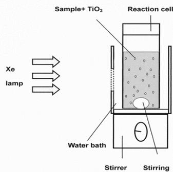
Figure 2: Photoreactor
