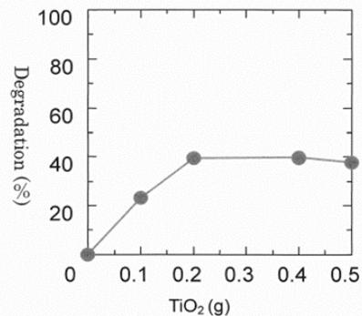
Figure 3: Effect of TiO<sub>2</sub> amount on photocatalytic degradation
